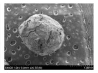
Fig. 13 SEM images of PLA-lignin coated urea pellets showing (a) the coating layer over urea core and the coated pellet (b) before and (c) after urea release to surrounding water. This figure has been adapted/reproduced from ref. 144 with permission from Elsevier B.V., copyright 2017.
