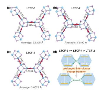
Fig. 4 Comparison between the three LTCFs in the distance between adjacent clusters (measured between Sn atomic center in linkers) (a-c). (d) Schematic diagram of intercluster charge transfer.
