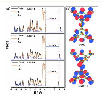
**Fig. 5** Theoretical calculations for LTCFs. (a) Theoretical band gaps calculated from DOS curves. (b) Distribution of excited states around LOMO in the structure of LTCFs.
