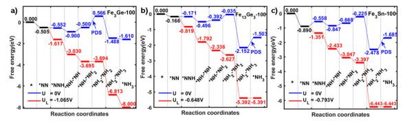
Fig. 4 Free energy diagrams of electrochemical nitrogen reduction on (a) Fe<sub>3</sub>Ge, (b) Fe<sub>13</sub>Ge<sub>3</sub> and (c) Fe<sub>3</sub>Sn, respectively. The best results among group-IV elements follow the sequence "Si > Ge > Sn".
