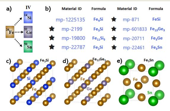
Fig. 1 (a): Fe-group-IVA binary alloys studied in this work. (b): Eight candidates of Fe-group-IVA binary alloys with their IDs and formulas from the Materials Project database. 54 (c-e): Conventional cells of some typical atomic structures among all studied candidates.
