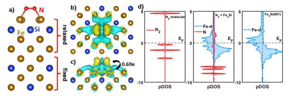
Fig. 2 (a): Horizontal mode of N<sub>2</sub> adsorption on the Fe<sub>3</sub>Si(100) surface. (b) and (c): Top and side views of the charge density difference plot of N<sub>2</sub> adsorption on the Fe<sub>3</sub>Si(100) surface. Yellow indicates charge accumulation and cyan represents charge depletion. The isosurface value is set to be 0.001 e Bohr<sup>-3</sup>. (d): Projected density of states (PDOS) of isolated N<sub>2</sub>, N<sub>2</sub> adsorbed Fe<sub>3</sub>Si, and Fe<sub>3</sub>Si.
