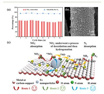
Fig. 4 (a) Nitrate conversion and nitrogen selectivity of Fe/GF during 8 repeated electrolysis tests. (b) SEM images of Fe/GF after 8 cycles. (c) Reaction mechanism diagram of Fe/metal or carbon support in the bielectrolyte (NaCl and Na<sub>2</sub>SO<sub>4</sub>) system.
