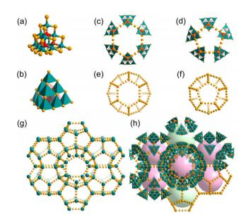
Fig. 1 Crystal structure of T3-MEP. (a and b) Discrete T3-like supertetrahedral cluster,  $[Sn_{10}O_4S_{20}]^{8-}$ , in ball-stick and polyhedral representation. (c and d) Hexagonal and pentagonal windows encircled by T3-clusters. (e and f)  $6^25^{12}$  cage A and  $5^{12}$  cage B created by connecting the centers of the supertetrahedral units. (g and h) MEP-type arrangement of the cluster anions and its MEP net topology. Sn, teal; S, gold; O, red.
