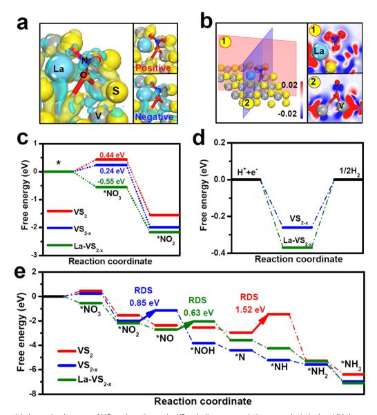
Fig. 4 (a) Differential charge density maps of  $NO_3^-$  adsorption on La-VS<sub>2-x</sub> (yellow: accumulation, cyan: depletion) and (b) the corresponding electron location function maps (red: accumulation, blue: depletion). (c and d) Binding free energies of (c)  $NO_3^-$  and (d) H on different catalysts. (e) Gibbs free energy diagrams of the  $NO_3RR$  pathway of  $VS_2$ ,  $VS_{2-x}$  and La- $VS_{2-x}$ , respectively.
