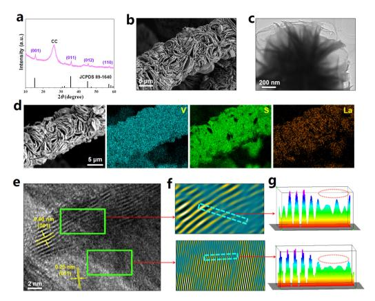
Fig. 1 (a) XRD pattern of La-VS<sub>2-x</sub> on CC. (b) SEM image of La-VS<sub>2-x</sub> on CC. (c) TEM image of La-VS<sub>2-x</sub>. (d) Elemental mapping images of La-VS<sub>2-x</sub> on CC. (e) HRTEM image of La-VS<sub>2-x</sub> and (f) the corresponding IFFT pattern and (g) lattice line scanning analyses.
