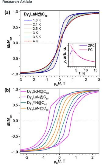
Fig. 7 (a) Magnetic hysteresis measurements for Dy<sub>2</sub>LaN@C<sub>80</sub> (magnetic field sweep rate: 2.9 mT s<sup>-1</sup>); the inset shows determination of  $T_B$ from FC/ZFC measurements. (b) Comparison of the magnetic hysteresis shape for  $Dy_2MN@C_{80}$  EMFs (M = Sc, Lu, Y, La) at 2 K (2.1 K for La); magnetic field sweep rate: 2.9 mT s<sup>-1</sup> for all compounds.
