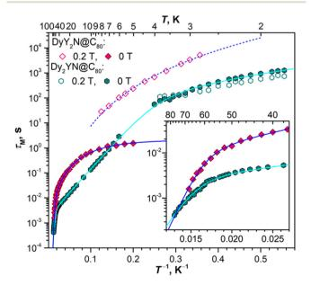
Fig. 9 Magnetization relaxation times of DyY2N@C80 and Dy2YN@C80 determined by DC and AC magnetometry (open points, at 0.2 T; filled points, at zero field). Lines are fits with relaxation mechanisms discussed in the text. The inset shows enlargement of the high-temperature part.
