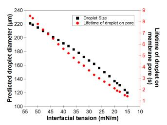
Fig. 4 Calculated relationship between the dynamic interfacial tension of a *n*-dodecane-water interface (from a bare interface to an equilibrium interfacial tension) in presence of PVA and the predicted droplet size formed at the membrane pore using eqn (3) and also the corresponding droplet lifetime before detachment from the membrane.
