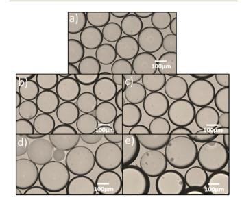
Fig. 6 Optical micrographs of n-dodecane droplets stabilised with 0.1 wt% aqueous solutions of mixed LMw-PVA-88 to HWw-PVA-88 at the following volume ratios; (a) 9:1, (b) 7:3, (c) 1:1, (d) 3:7 and (e) 1:9. The images show changes in the droplet size and more importantly the droplet uniformity at the different polymer blend ratios. The stirred paddle rotational speed and the dispersed phase injection rate was kept constant at 1000 rpm and 0.1 mL min<sup>-1</sup> respectively.
