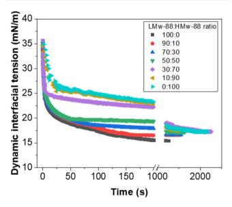
Fig. 7 Long term dynamic interfacial tension measurements of an n-dodecane-water interface in the presence of different volume ratios of LMw-PVA-88: HMw-PVA-88 polymer. Each polymer mixture was prepared at a total polymer concentration of 0.1 wt% and all measurements were conducted at 20 °C
