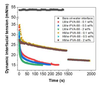
Fig. 3 Dynamic interfacial tension of a *n*-dodecane—water interface in the presence of LMw-PVA-88 and HMw-PVA-88 polymer at different polymer concentrations. For reference the interfacial tension of a bare *n*-dodecane—water interface is also presented. All measurements were conducted at 20 °C.
