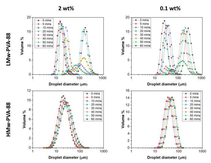
Fig. 1 Evolution of the droplet size and size distribution of *n*-dodecane in water emulsions produced using an Ultra-Turrax homogeniser operated at 12 000 rpm for 2 minutes over time, measured by laser diffraction These emulsions were designed with a dispersed phase volume of 10% and stabilised by 88% hydrolysed PVA at 2 different molecular weights (LMw-PVA-88 and HMw-PVA-88) and at two different polymer concentrations (0.1 and 2 wt%)
