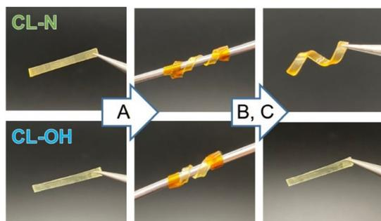
**Fig. 4** Difference of reprocessability between CL-N and CL-OH during the process with A: fixing the sample with kapton tapes, B: heating in an oven ( $150 \text{ }^\circ\text{C}$ , 30 min), and C: cooling to  $25 \text{ }^\circ\text{C}$  (room temperature).
