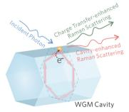
Fig. 3 Schematics of the proposed WGM sensing mechanisms. The charge transfer and cavity effect both contribute to the overall Raman intensity enhancement.
