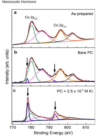
Fig. 5 X-ray photoelectron spectra of Co  $2p_{1/2}$  and Co  $2p_{3/2}$  for (a) asprepared, (b) treated in bare PC and (c) PC +  $2.5 \times 10^{-4}$  M KI samples. The downward arrows point to the Co  $2p_{3/2}$  and Co  $2p_{1/2}$  peaks of metallic Co (in blue and purple in (b) and (c)). Additionally, green and orange correspond to Co<sup>2+</sup>, and pink and brown to Co<sup>3+</sup>. Solid black lines are experimental data, whereas solid red lines refer to fitting spectra.
