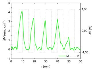
Fig. 6 Magneto-ionic cyclability of the 15 nm-thick cobalt oxide film in PC with  $2.5 \times 10^{-4}$  M KI under -1.35 V/+1.35 V voltage pulses of 10 min duration each, assessed from in-plane magnetic measurements while applying a magnetic field of 10 kOe.
