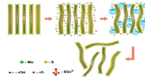
Fig. 7 (a) Schematic illustration of the experimental setup for the anodic electrochemical exfoliation of bulk  $MoS_2$  crystal. (b) Schematic diagram of the electrochemical setup for exfoliation of natural  $MoS_2$  crystals. (c) Schematic illustration of the electrochemical exfoliation mechanism. Adapted with permission from ref. 65 (ACS Nano, 2014, 8(7), 6902–6910) Copyright (2014) American Chemical Society.
