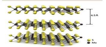
Fig. 2 Crystalline structure of MoS<sub>2</sub>, adapted from ref. 2 from Springer Nature, copyright 2014 (Owned by Springer Nature).
