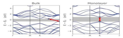
Energy band structure diagrams of bulk and monolayer MoS<sub>2</sub>. Adapted from ref. 4 with permission from MDPI, copyright 2022.
