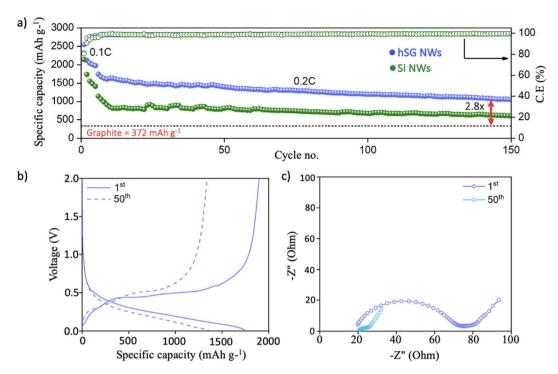
Fig. 3 (a) Cyclic performance of hSG NWs and Si NWs at 0.2C cycled between 0.011-2.0 V, (b) corresponding voltage-specific capacity plot and (c) EIS analysis of hSG NWs after 1<sup>st</sup> and 50<sup>th</sup> cycle of hSG NWs.
