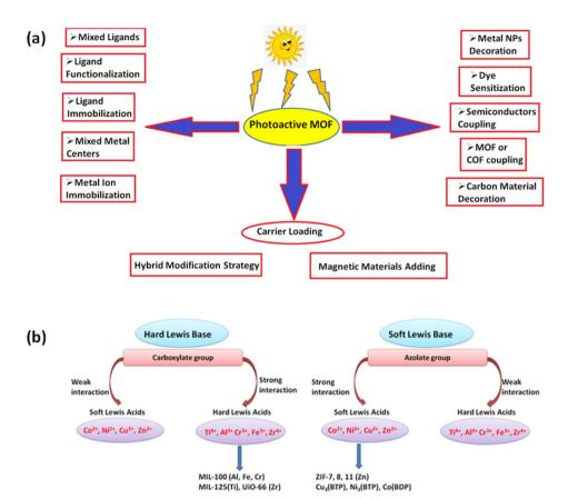
Fig. 6 (a) Strategies to engineer MOFs as efficient photocatalysts for environmental applications; (b) strategies to construct stable MOFs by carboxylate and azolate groups guided by HSAB theory.
