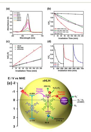
Fig. 7 (a) Absorption spectra of Rh B solution in the presence of H<sub>2</sub>O<sub>2</sub> and nMLM; (b) visible-light photocatalytic degradation curve of Rh B over nMLM, nPCN-222, and nNU-1000; (c) kinetic study of the degradation process over nMLM, nPCN-222, and nNU-1000; (d) recycling test for nMLM; (e) proposed mechanism for rhodamine B (Rh B) degradation using nMLM.<sup>157</sup> This figure has been adapted from ref. 157 with permission from American Chemical Society, copyright 2020.
