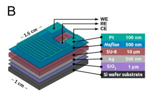
Fig. 4 (A) Electrochemical methane sensing using IL-based electrolytes. CO<sub>2</sub> generated by successive methane oxidation on the WE, and active oxygen species were used as an internal standard. 162 Adapted with permission from ref. 162 Copyright 2014 Royal Society of Chemistry. (B) Scheme showing a multilayered electrochemical device based on solid-state electrolyte Nafion for methane sensing. 161 Reprinted with permission from ref. 161 Copyright 2018 American Chemical Society.
