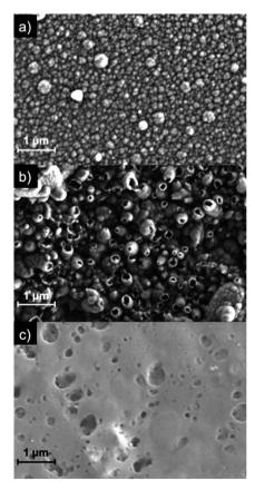
Fig. 5 SEM images of PPy grown to a charge density of 210 mC cm $^{-2}$  onto (a) Au and (b) PSI/Au. A drop-cast film of PSI (no Ppy) is shown in (c) as a comparison.
