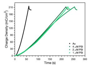
Fig. 4 Time dependence of PPy growth on Au as quantified through charge density in the absence and presence of a PSI film. A 40  $\mu$ L drop of PSI solution at the given concentrations was drop-cast for each film to vary the amount of PSI on the Au substrate. The applied voltage was 0.65 V vs. Ag/AgCl.
