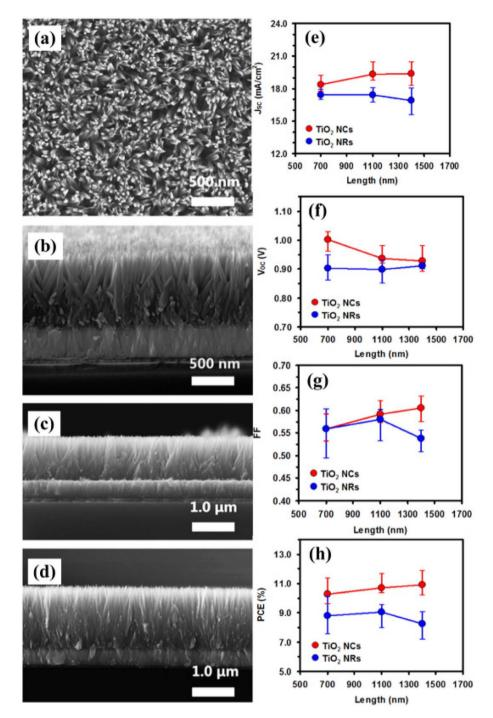
Fig. 12 (a) Top view of nanocones and (b) side view of SEM image of  $TiO_2$  nanocones grown over FTO glass substrate (a and b) with 700 nm, (c) 1100 nm, (d) 1400 nm,  $TiO_2$  nanocones. Comparative works of both  $TiO_2$  nanocones and nanorods for 16 devices having various physical parameters (e)  $J_{SC}$ , (f)  $V_{OC}$ , (g) FF, and (h) PCE of PSCs with respect to length (reproduced with permission from ref. 139. Copyright 2015 Elsevier).
