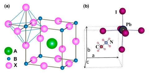
Fig. 1 (a)  $ABX_3$  perovskite construction presenting  $BX_6$  octahedral and bigger A cations engaged in the cuboctahedral place. (b) The element cell of cubic MAPbl<sub>3</sub> perovskite (reproduced with permission from ref. 25, copyright 2015 Elsevier).
