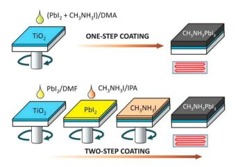
Fig. 23 One-stage and two-stage coating methods to prepare CH<sub>3</sub>-NH<sub>3</sub>Pbl<sub>3</sub> perovskite layers. DMA, DMF, and IPA signify dimethyl acetamide, dimethyl formamide, and isopropyl alcohol, respectively (reproduced with permission from ref. 197. Copyright 2014 AIP).
