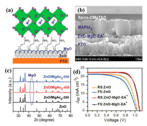
Fig. 14 (a) Graphic depiction of altered planar perovskite thin-film assembly with ZnO-MgO-EA<sup>+</sup>. (b) SEM image exhibiting the side view of the device. (c) XRD arrangement of the precursor solution having diverse temperature environments. (d)  $J_{SC}$ -V curves. (Reproduced with permission from ref. 147, Copyright 2018 Wiley-VCH).
