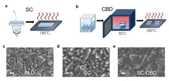
Fig. 22 Symbolic diagram showing the preparation of  $SnO_2$  thin layers using (a) spin coating (SC) and (b) chemical bath deposition (CBD). (c) Top-view SEM pictures of  $SnO_2$  films prepared by atomic layer deposition (ALD), (d) spin coating (SC), and (e) spin coating and chemical bath deposition (SC-CBD). All scale bars are 200 nm (reproduced with permission from ref. 74. Copyright 2016 RSC).
