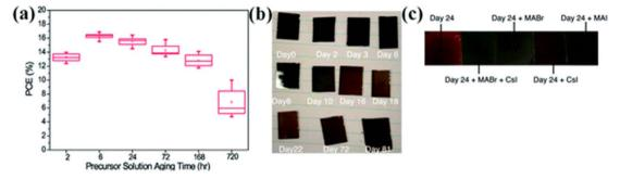
Fig. 29 (a) PCE distribution with precursor solution aging time (hours) of the triple-cation lead halide PSCs.<sup>223</sup> (b) Photographs of triple-cation (FA, MA, Cs) films produced from fresh ink (*viz.*, 0 days of storage, labeled as "Day 0") and the same ink is utilized for the 2–81 days storage. (c) Snapshots of layers made up from 24 days old ink. (Reproduced with permission from ref. 224. Copyright 2020 ACS).
