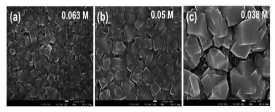
Fig. 24 SEM images for CH<sub>3</sub>NH<sub>3</sub>Pbl<sub>3</sub> produced *via* two-step spin-coating with (a) 0.063 M, (b) 0.05 M, and (c) 0.038 M CH<sub>3</sub>NH<sub>3</sub>I solution. Scale bars signify 100 nm (reproduced with permission from ref. 200. Copyright 2014 NPG).
