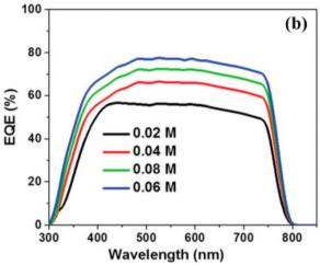
Fig. 13 (a) J-V, and (b) EQE properties of PSCs as a function of precursor concentration 0.02 M, 0.04 M, 0.08 M, 0.06 M (reproduced with permission from ref. 145. Copyright 2014 RSC).
