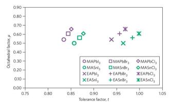
Fig. 2 Tolerance factor (t) and octahedral factor ( $\mu$ ) calculated values for perovskites (reproduced with permission from ref. 28, copyright 2014 NPG).
