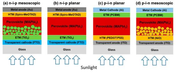
Fig. 4 Diagram displaying the four-layered assemblies of PSCs (a) n-i-p mesoscopic, (b) n-i-p planar, (c) p-i-n planar, and (d) p-i-n mesostructured (reproduced with permission from ref. 36, copyright 2016 SPIE).
