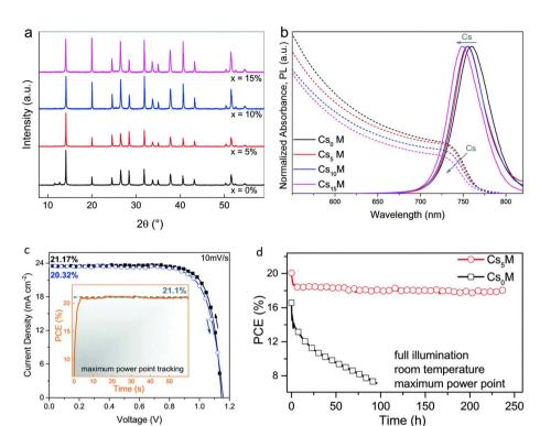
Fig. 8 Consequences of Cs accumulation in MA/FA cation blends; (a) XRD and (b) optical findings (c) current–voltage (J-V) and (d) stability properties of Cs<sub>x</sub>MAFA complexes (reproduced with permission from ref. 60. Copyright 2017 RSC).
