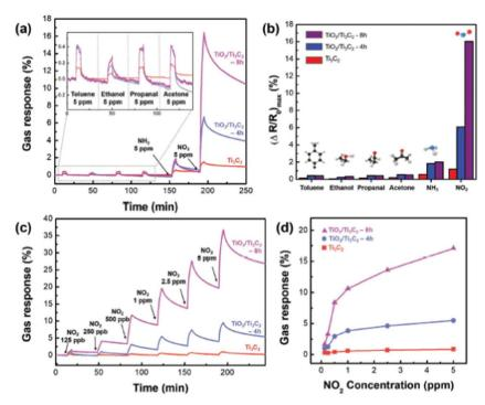
Fig. 12 (a) Selective response to gas and (b) maximum change in resistance when exposed to 5 ppm of toluene, ethanol, propanol, acetone,  $NH_3^+$ , and  $NO_2$ . (c) The  $TiO_2/Ti_3C_2$  real-time gas response curve as a function of  $NO_2$  concentration and (d) graph showing maximal resistance change dot at room temperature ( $NO_2$ , at concentrations ranging from 0.125 to 5 ppm), reprinted in part permission from ref. 93 from Copyright (2023) Wiley materials.
