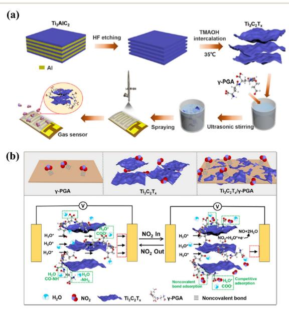
Fig. 11 Techniques used to improve the  $NO_2$  sensing performance of  $Ti_3C_2T_x$  by modifying with  $\gamma$ -poly( $\iota$ -glutamic acid): (a) schematic representation of the fabrication of oligo-layer  $Ti_3C_2T_x$  and deposition of the  $Ti_3C_2T_x/\gamma$ -PGA nanocomposite film. (b) Gas sensor's NO<sub>2</sub> gassensing mechanism, reprinted with reprinted in part permission from ref. 51 from Copyright (2023) American Chemical Society.
