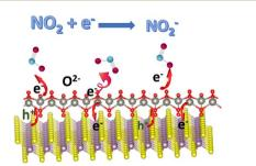
Fig. 3 NO<sub>2</sub> sensing mechanism based on an ionosorption model for 2D materials.
