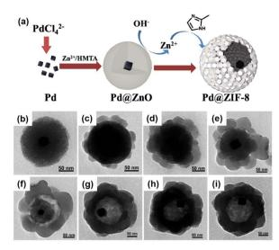
Fig. 4 (a) Schematic illustration of the fabrication of yolk-shell Pd-NPNS@ZIF-8 nanoparticles via the self-template approach, (b) TEM image of core-shell Pd@ZnO nanoparticles, and (c-i) time-resolved TEM images illustrating the structural evolution of yolk-shell Pd-NPNS@ZIF-8 nanoparticles as a function of reaction time: (c) 5 min, (d) 10 min, (e) 20 min, (f) 30 min, (g) 60 min, (h) 120 min, and (i) 240 min (Copyright 2016, Royal Society of Chemistry).45
