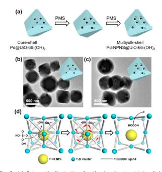
Fig. 9 (a) Schematic illustration for the localized oxidative linker cleaving process; (b and c) TEM images of (b) core-shell Pd@UiO-66-(OH)<sub>2</sub> and (c) multiyolk-shell NPNS@MOF nanostructures; (d) schematic illustration of the oxidative linker cleaving process catalyzed by Pd nanoparticles in core-shell Pd@UiO-66-(OH)2 nanoparticles (abbreviations: PMS = peroxymonosulfate; DOBDC = 2,5-dihydroxyterephthalic acid) (Copyright 2019, American Chemical Society).60
