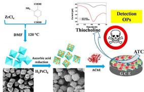
Fig. 15 Schematic representation of detection of organophosphates using Pt@UiO-66-NH<sub>2</sub>@GCE (reproduced with permission from Li Ma et al.<sup>97</sup> Copyright 2019 Elsevier).
