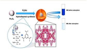
Fig. 7 Schematic representation of the *in situ* one-step hydrothermal synthesis of  $Fe_3O_4@MIL-100(Fe)$  core—shell magnetic microspheres (reproduced with permission from ref. 45. Copyright 2017 Elsevier).
