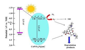
Fig. 11 Schematic illustration of the photodegradation process of RhB over the CoP/Fe<sub>2</sub>P@mC nanocomposites (reproduced with permission from ref. 70. Copyright 2018 Elsevier).
