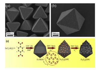
Fig. 10 SEM images of (a) Fe-MOF crystals, (b) single Fe-MOF crystal, (c) schematic representation for the synthesis of nanocomposite Fe<sub>3</sub>O<sub>4</sub>@NPC derived from Fe-MOF. Reproduced with permission from ref. 58. Copyright 2019 Springer.
