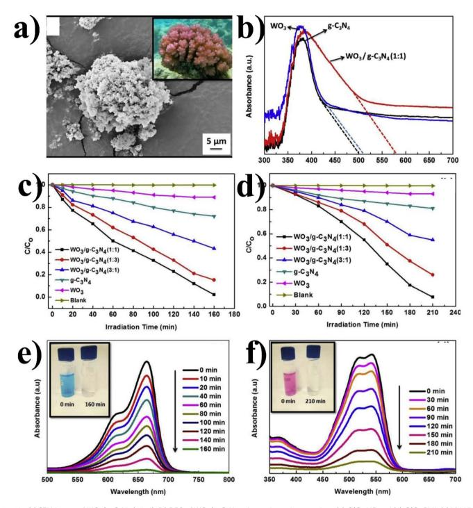
Fig. 12 (a) SEM image of  $WO_3/g-C_3N_4$  (-1:1), (b) DRS of  $WO_3/g-C_3N_4$  using various photocatalysts (c)  $C/C_0$  MB and (d)  $C/C_0$  RbX. (e) UV-Vis spectra at different time intervals under visible light for the degradation of MB and (f) RbX using  $WO_3/g-C_3N_4$  (-1:1) (reproduced with permission from ref. 120 Copyright 2019, Elsevier).
