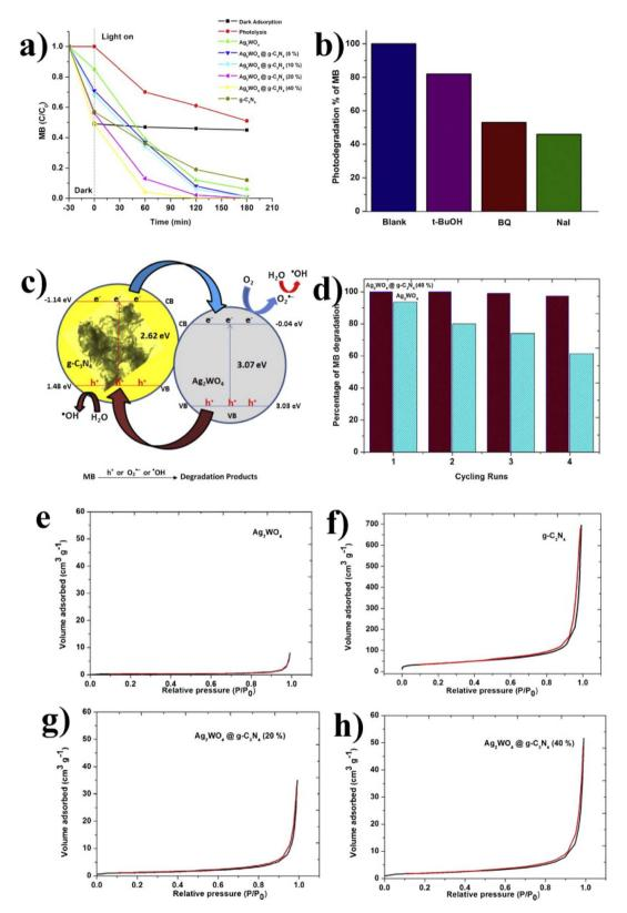
Fig. 14 (a)  $C/C_0$  MB (10 ppm); (b) schematic diagram of electron–hole transfer. (c) Influence of radical scavengers on MB. (d) Cycling runs. (e–h) The N<sub>2</sub> adsorption/desorption isotherms of the pristine  $Ag_2WO_4$ ,  $g-C_3N_4$ , and  $Ag_2WO_4$ @ $g-C_3N_4$  composite (reproduced with permission from ref. 41 Copyright 2015, Elsevier).
