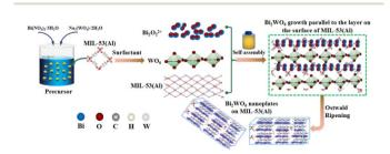
Fig. 3 The formation mechanism of BWO/MIL.
