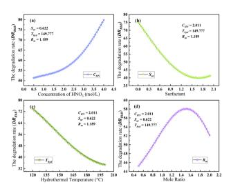
Fig. 9 SA of the four features based on the SVR-RBF model (a)  $C_{HN}$ , (b)  $S_{\rm ur}$ , (c)  $T_{\rm hyd}$  and (d)  $R_{\rm m}$ .
