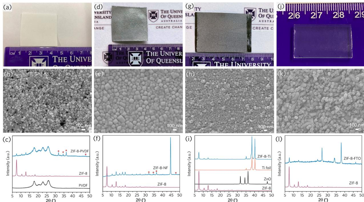
**Fig. 9** Mechanochemical coating of ZIF-8 on various substrates: (a–c) one-pot coating on PVDF from ZIF-8 precursors, (d–f) one-pot coating on nickel foam (NF) from ZIF-8 precursors, (g–i) one-pot coating on Ti foils from ZIF-8 precursors, (j–l) ZIF-8 coating on FTO glass. Reproduced with permission from ref. 2.
