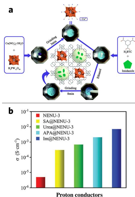
**Fig. 11** (a) Schematic procedure of mechanochemically synthesized IM/MOF composite (b) the comparison of proton conductivity of the guest@NENU-3 composite and NENU-3 @338k. Reproduced with permission from ref. 1.
