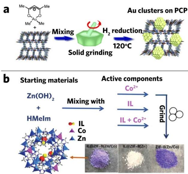
Fig. 10 (a) Mechanochemical deposition of gold clusters on porous coordination polymers. Reproduced with permission from ref. 100, (b) synthetic procedures of L@ZIF-8(Zn/Co). Reproduced with permission from ref. 133.
