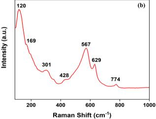
Fig. 2 (a) FTIR spectra and (b) Raman spectra of SnO<sub>2</sub> NPs.
