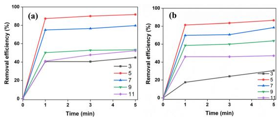
Fig. 7 Effect of pH on removal efficiency for two dye concentrations: (a) 5  $\mu$ M and (b) 10  $\mu$ M.
