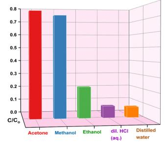
Fig. 11 Bar diagram showing the concentration of desorbed Congo red in various eluents from the adsorbent.
