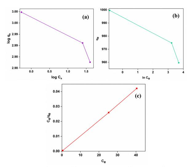
Fig. 9 Adsorption isotherms for 5  $\mu$ M CR adsorption by SnO<sub>2</sub> at pH = 5 and room temperature. (a) Freundlich isotherm, (b) Temkin isotherm and (c) Langmuir isotherm.
