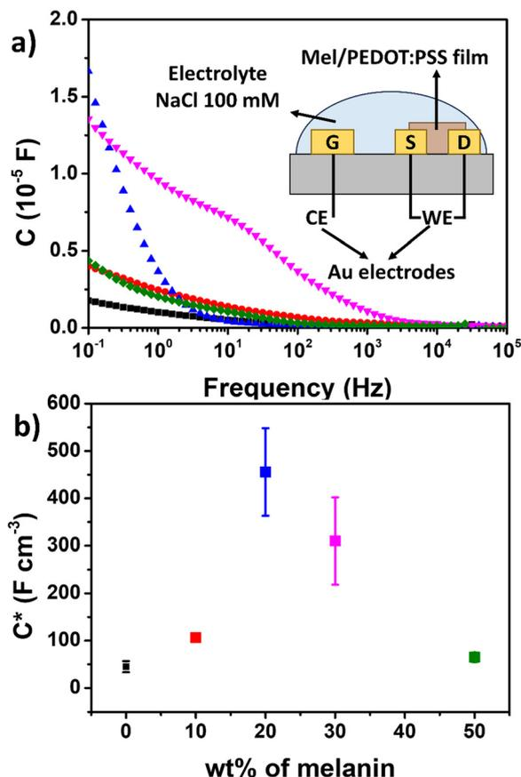
Fig. 5 EIS characterization of Mel/PEDOT:PSS films. (a) capacitance as a function of frequency (inset: scheme of 2-electrode configuration measurement). (b) volumetric capacitance ( $C^*$ ) as a function of wt% Mel in PEDOT:PSS matrix.
