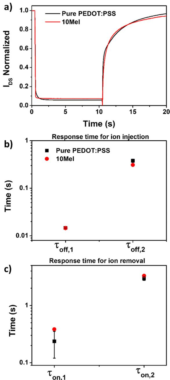
Fig. 7 Response time of OECTs. (a) Normalized  $I_{DS}$ -time curve for OECTs employing 10 Mel and pure PEDOT:PSS films upon application of a single positive  $V_{GS}$  bias +0.8 V (pulse width = 10 s) at fixed  $V_{DS} = -0.6$  V, and  $V_{GS} = 0$  V. Corresponding time constants ( $\tau$ ) for the (b)  $I_{DS}$  decay and (c)  $I_{DS}$  growth using a double exponential function.
