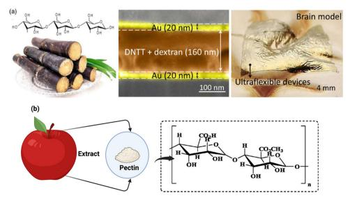
Fig. 4 Biomaterial-based artificial synaptic devices with ultraflexibility: (a) ultraflexible organic synaptic transistors based on dextran; 48-50 (b) organic synaptic transistors based on pectin from apples
