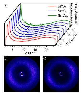
**Fig. 6** (a) Temperature dependent WAXS measurements of **16O-AzCN-PhO8**. (b) 2D diffractogram of the WAXS measurement of the SmA phase at  $T-T_{\rm AC}=20$  K and (c) of the SmA $_{\rm re}$  phase at  $T-T_{\rm AC}=-50$  K.
