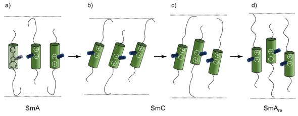
Fig. 9 Proposed mechanism for the formation of the SmA<sub>re</sub> phase of **160-AzCN-PhO8** due to a shift of mass centers based on a model by Novotná et al. 14 (a) The SmA phase is present. (b) Tilting of the mesogens in the SmC phase leads to layer contraction. (c) A shift of mass centers is induced by the hindrance of the nitrile group and the layer thickness increases. (d) Mesogens lose their tilt in the SmA<sub>re</sub> phase, the layer thickness further increases.
