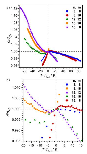
Fig. 5 Plot of the relative layer spacing  $d/d_{\rm AC}$  as a function of  $T-T_{\rm AC}$  for  ${\it nO-AzCN-PhOm}$ . (a) Full size and (b) close to the SmA-C transition.
