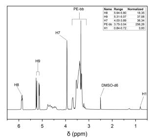
Fig. 2 <sup>1</sup>H NMR spectrum of hPG-co-AGE used for structural characterization.
