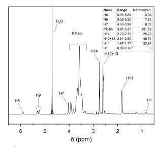
Fig. 3 <sup>1</sup>H NMR spectrum of hPG-NH<sub>2</sub> used for structural characterization.
