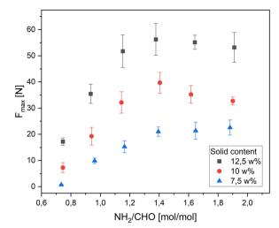
Fig. 6 Hydrogel stability depending on the amine to aldehyde ratio.
