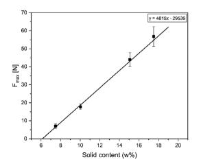
Fig. 5 Hydrogel stability depending on the solid content.
