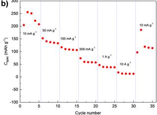
**Fig. 7** Electrochemical performance of **D-PTO-2a** based composite electrodes within the potential range of  $1.5-4~V~(vs.~Li/Li^+)$ : (a) cycling performance at  $100~mA~g^{-1}$ . (b) Rate performance at various current densities.
