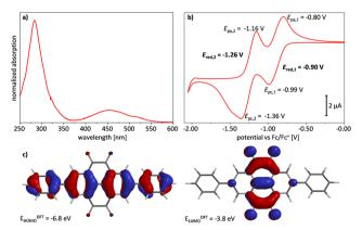
Fig. 2 (a) UV/Vis spectrum of compound 2 measured in  $CH_2Cl_2$  at rt (1  $\mu$ mol L<sup>-1</sup>). (b) Cyclic voltammogram of model compound **2** (CH<sub>2</sub>Cl<sub>2</sub>, nBu<sub>4</sub>NPF<sub>6</sub> (0.1 M), measured at rt with Pt-working electrode and (Fc/Fc+) as internal reference, scanning velocity: 100 mV  $s^{-1}$ ). (c) DFT model (B3LYP: 6-311++G\*\*) of compound 2 (tert-butyl groups omitted).
