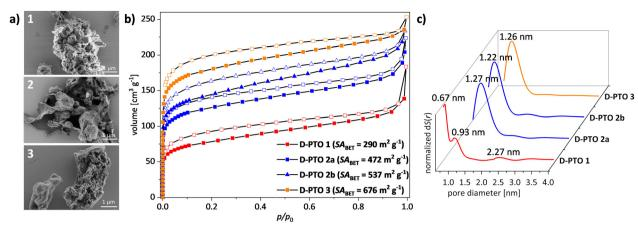
Fig. 5 (a) SEM images of **D-PTO-1**, **-2a**, and **-3** (from top to bottom). (b) BET gas sorption isotherms (N<sub>2</sub>, 77 K, vector dosing) after activation at 120 °C for 12 h. (c) pore size distribution (QSDFT, Kernel: N<sub>2</sub> on carbon at 77 K, sphere/cylindrical pore.
