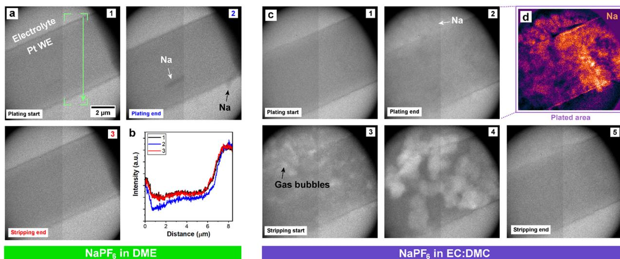
Fig. 2 Operando electrochemical liquid-cell TEM imaging. (a) Galvanostatic cycle ( $10 \text{ mA cm}^{-2}$ ) of  $\text{NaPF}_6$  in DME. Annotation in panel 1 denotes where box-averaged intensity profiles were acquired from each panel. (b) Intensity profiles extracted from panels 1 to 3. (c) Galvanostatic cycle ( $10 \text{ mA cm}^{-2}$ ) of  $\text{NaPF}_6$  in EC:DMC. (d) False-color look-up table of panel 2 following background subtraction, highlighting Na deposition.
