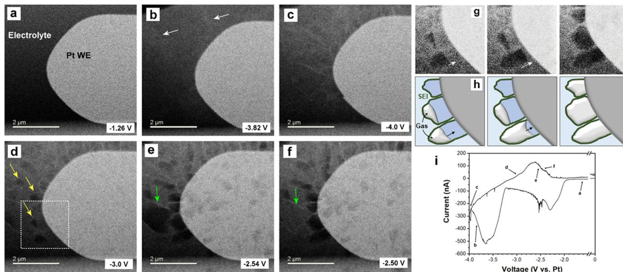
Fig. 3 Operando electrochemical HAADF-STEM imaging of bubble formation from 1 M NaPF<sub>6</sub> in EC:DMC with 10% FEC. (a–f) Liquid-cell STEM time-series of cyclic voltammetry cycling showing Na plating and stripping. (g) Magnified views showing bubble formation during stripping. (h) Illustrations corresponding to (g). (i) Cyclic voltammetry profile corresponding to panels (a–f).
