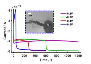
Fig. 3 i vs. t plots recorded during the potentiostatic ( $E_{app} = -0.20$  -(-0.50) V) single-barrel SECCM eATRP/FRP of Am using [Am]: [HEBiB]:  $[Cu^{II}]$ : [TPMA] = [20]: [1]: [0.5]: [0.625]; (inset) SEM image of a gel-like feature formed when  $E_{app} = -0.50 \text{ V}$ .
