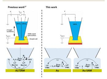
Fig. 1 Schematic showing the operationally complex dual-barrel SECCM configuration and Cu/Me<sub>6</sub>Tren as a catalyst for localised eATRP which was found to proceed with a competing undesirable ROS-initiated mechanism (left). 17 Here we employ simplified single-barrel SECCM for the first time to control eATRP both at and from the surface of a gold electrode (right)
