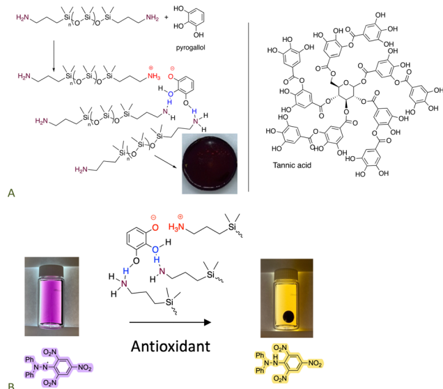
Fig. 13 (A) Formation of elastomers simply by mixing aminosilanes with phenols. (B) Antioxidant activity of the elastomer formed. 70 Photographs from ref. 70 reproduced with permission from the American Chemical Society.
