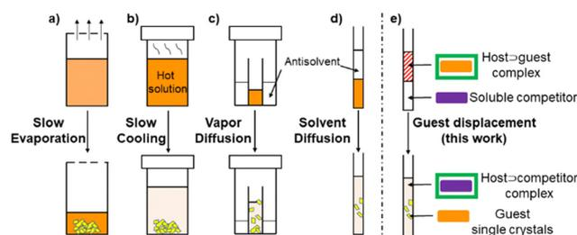
**Fig. 1** Various methods used to grow single crystals from solution. (a) Slow evaporation of solvent, (b) slow cooling of a hot solution, (c) vapor diffusion of an antisolvent using a saturated solution of the analyte, (d) diffusion of an antisolvent layered on top of the analyte solution, and (e) displacement of the guest encapsulated in a soluble macrocyclic host by a competitor (this work).
