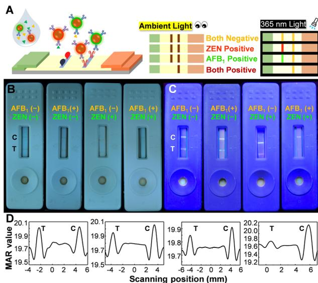
**Fig. 2** (A) A diagram illustrating the production process of multiplexed ICTS for co-detection of ZEN and AFB<sub>1</sub>. (B) Photographs of test strips after interacting with sample solutions containing varying concentrations of AFB<sub>1</sub> and ZEN. Their corresponding (C) fluorescence images under UV light and (D) magnetic signals. The AFB<sub>1</sub>/ZEN concentrations in (B–D) are as follows (from left to right): 0/0, 150/0, 0/150, 150/150 ng mL<sup>-1</sup>.
