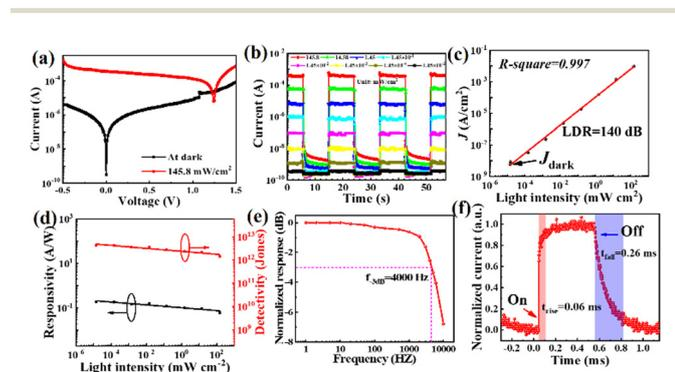
Fig. 4 The performance of the CsPbBr<sub>3</sub> nanonet PD with the optimal BMIMBr ionic liquid concentration (1 mg mL<sup>-1</sup>): (a) *I*-*V* curves; (b) *I*-*t* curves at different light intensities; (c) LDR; (d) *R* and *D*\*; (e) *f*<sub>-3dB</sub> bandwidth; (f) response speed.
