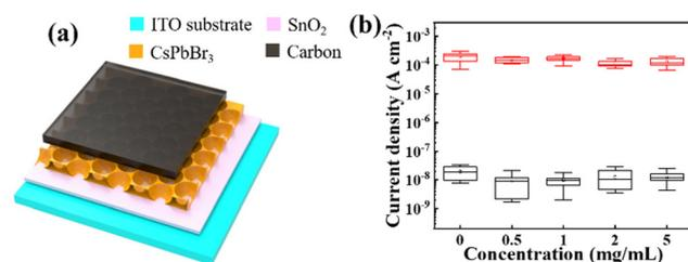
Fig. 3 (a) Schematic structure of the CsPbBr<sub>3</sub> nanonet PD. (b) Light and dark current statistics of the CsPbBr<sub>3</sub> nanonet PDs with various concentrations of BMIMBr ionic liquid.
