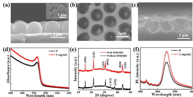
Fig. 2 (a) Cross-sectional SEM image of single-layer PS spheres; the inset shows the top view SEM image of single-layer PS spheres. Top (b) and cross-sectional (c) SEM image of the CsPbBr<sub>3</sub> perovskite nanonet film with BMIMBr ionic liquid. (d) Absorption spectra of the CsPbBr<sub>3</sub> perovskite nanonet films. (e) XRD patterns of the CsPbBr<sub>3</sub> perovskite nanonet films. (f) Steady-state PL spectra of the CsPbBr<sub>3</sub> perovskite nanonet films.
