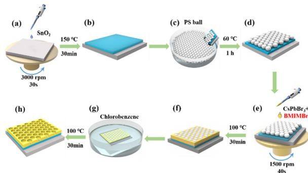
Fig. 1 Schematic diagram of the fabrication process for the CsPbBr<sub>3</sub> perovskite nanonet.
