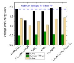
Fig. 2 Optical bandgap, experimentally obtained  $V_{\rm OC}$ , and voltage losses of PIM-based IPVs.
