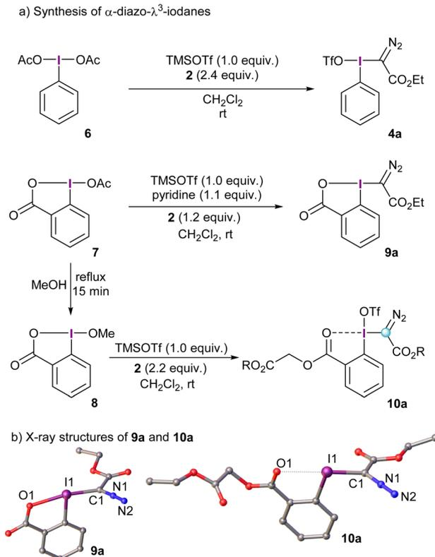
Scheme 2 Synthetic pathways towards  $\alpha$ -diazo reagents **4a**, **9a** and **10a** and X-ray structures of **9a** and **10a**. Hydrogen atoms and triflate-anion (**10a**) omitted for clarity; ellipsoids shown at 50% probability level.
