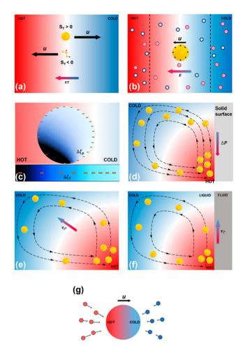
**Fig. 2** Schematics of physical mechanisms for heat-mediated optical manipulation: (a) thermophoresis, (b) thermoelectricity, (c) thermoelectrokinetics, (d) thermo-osmosis, (e) thermal convection, (f) thermocapillarity, and (g) photophoresis. Adapted with permission.<sup>37</sup> Copyright 2022, American Chemical Society.
