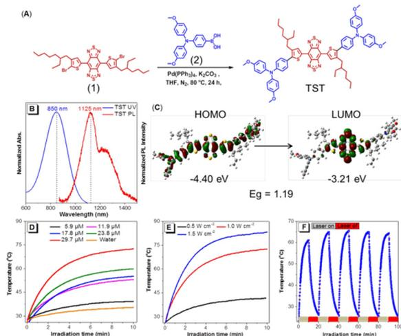
Fig. 2 (A) Synthetic route to TST. (B) Normalized absorption and photoluminescence spectra of TST in THF. Concentration of TST: 10  $\mu\text{M}$ ;  $\lambda_{\text{ex}}$ : 850 nm. (C) HOMO and LUMO distribution and the energy states of TST. (D) and (E) Heating curves of TST NPs with different concentration and laser power, respectively. (F) Photothermal stability of TST NPs under 808 nm laser ( $1 \text{ W cm}^{-2}$  for 10 min) irradiation with five heating/cooling cycles.
