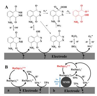
Fig. 2 Schematic representation of ECL mechanisms. (A) Homogeneous, luminol-H<sub>2</sub>O<sub>2</sub> system; (B) homogeneous (a), heterogeneous (b),  $Ru(bpy)_3^{2+}$ -TPA system.
