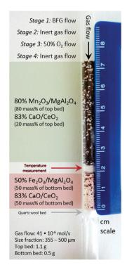
Fig. 3 Laboratory reactor bed to carry out the proof of concept experiments and experimental specifications. The scale bar on the right indicates the length in cm. Gas flow:  $41 \times 10^{-6}$  mol s<sup>-1</sup>. Size fraction of solids: 355– 500 μm. Top bed (manganese oxide and calcium oxide): 1.1 g. Bottom bed (iron oxide and calcium oxide): 0.5 g
