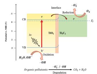
Fig. 9 Schematic diagram of charge transfer and photocatalytic degradation mechanisms via the TiO<sub>2</sub>/Ti<sub>3</sub>C<sub>2</sub> heterojunction.
