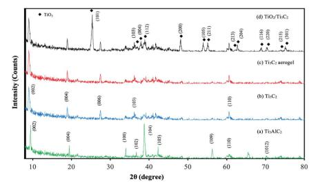
Fig. 1 XRD spectra of Ti<sub>3</sub>AlC<sub>2</sub>, Ti<sub>3</sub>C<sub>2</sub> nanosheet, Ti<sub>3</sub>C<sub>2</sub> aerogel and TiO<sub>2</sub>/Ti<sub>3</sub>C<sub>2</sub> aerogel composite.
