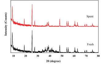
Fig. 8 XRD spectra of fresh and spent  $TiO_2/Ti_3C_2$  MXene aerogel composites.
