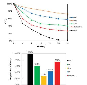
Fig. 10 Effect of radical scavengers on the POME degradation efficiency using the {001}-TiO<sub>2</sub>/Ti<sub>3</sub>C<sub>2</sub> aerogel composite.
