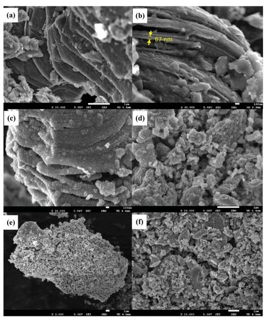
Fig. 3 FESEM images of (a and b) Ti<sub>3</sub>C<sub>2</sub> MXene, (c and d) Ti<sub>3</sub>C<sub>2</sub> MXene aerogel, and (e and f) TiO<sub>2</sub>/Ti<sub>3</sub>C<sub>2</sub> MXene aerogel composite.
