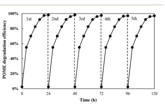
Fig. 7 Photostability test of the  ${\rm TiO_2/Ti_3C_2}$  MXene aerogel composite for POME degradation.
