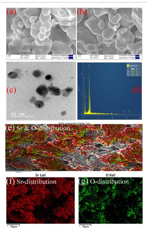
Fig. 2 (a and b) FE-SEM images of bio-synthesized SrO NPs, (c) TEM image of bio-synthesized SrO NPs, (d) EDX spectrum of SrO NPs. (e-g) Mapping images of synthesized SrO NPs.
