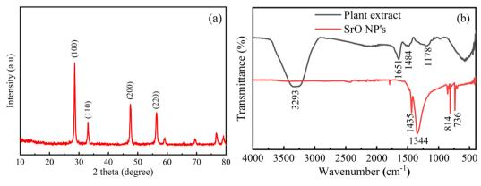
Fig. 1 (a) X-ray diffraction pattern of biosynthesized SrO NPs. (b) FTIR spectra of Albizia julibrissin extract and SrO NPs
