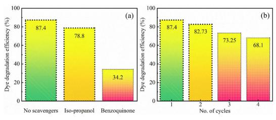
Fig. 7 (a) Dye degradation efficiency in the presence of scavengers and (b) reusability of the SrO sample under visible-light irradiation (irradiation time 80 min).
