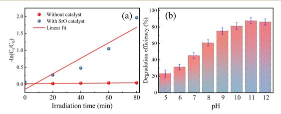
Fig. 6 (a) Kinetics of the degradation reaction for MB dye in the presence and absence of SrO nanoparticles and (b) effect of pH on the degradation of MB in the presence of SrO (irradiation time 80 min). Error bars indicate the % error in the repeated experiments.
