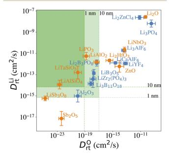
Fig. 4 Calculated room-temperature self-diffusion coefficients of Li<sup>+</sup>  $(D_{\rm rt}^{\rm Li})$  and  ${\rm O}^{2-}$   $(D_{\rm rt}^{\rm O})$  in the selected compounds. The dash lines represent the approximated  $D_{rt}^{Li}$  and  $D_{rt}^{O}$  limits based on a coating thickness between 1 to 10 nm.
