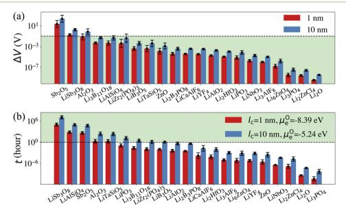
Fig. 5 (a) Calculated overpotentials ( $\Delta V$ ) for a current density of 0.044 mA cm<sup>-2</sup> across room temperature cathode coatings of  $l_c = 1$  and 10 nm. The dashed line represents  $\Delta V = 0.1 \, \text{V}$ . (b) Calculated O<sup>2-</sup> diffusion time t in the selected compounds assuming an  $r = 1 \, \mu \text{m}$  primary particle and an  $l_s = 2$  nm surface rocksalt phase. The dashed line represents t = 1 h.
