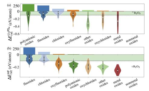
Fig. 3 Distribution of the reaction energy  $\Delta E_{rxt}$  with Li<sub>3</sub>PS<sub>4</sub> (a) and HF (b) for each category that pass chemical stability with the cathodes descriptor. The horizontal dash lines represent the limits of the descriptors. The histograms in (a) and (b) illustrate the numbers of compounds for each category that pass the descriptors.
