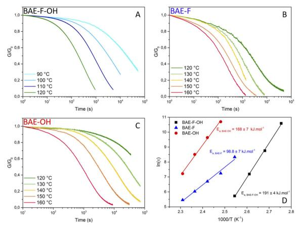
Fig. 4 Normalized stress-relaxation curves at different temperatures for a 1% strain (A) for BAE-F-OH, (B) for BAE-F and (C) for BAE-O. (D) Fitting of the relaxation time (τ) vs. temperature data by the Arrhenius equation for BAE-F-OH (black squares), BAE-F (blue triangle) and BAE-OH (red circles).
