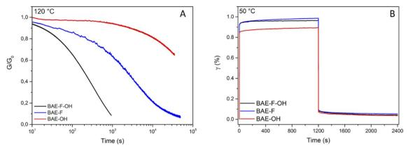
(A) Normalized stress relaxation of BAEs at 120 °C for a 1% strain (B) creep and recovery data for BAEs at 50 °C for an applied stress of 2 kPa.
