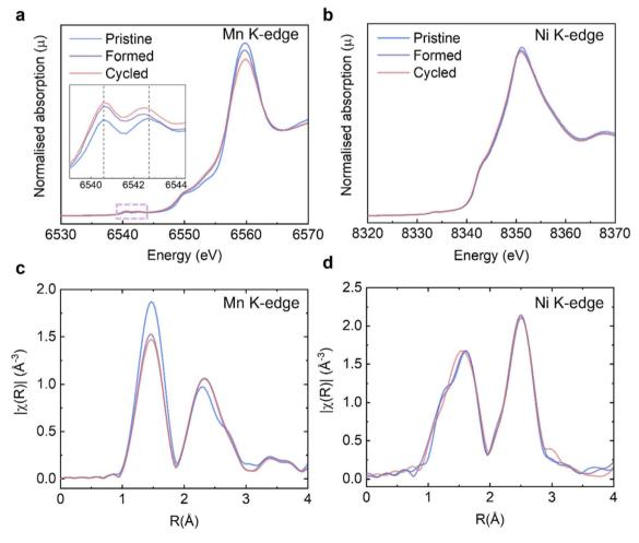
Fig. 5 XAS analysis on  $Li_{1.2}Ni_{0.2}Mn_{0.6}O_2$  structural changes. Evolution of XANES at the (a) Mn; (b) Ni K-edges. Inset in (a) shows an enlargement of the pre-edge features. Evolution of EXAFS at the (c) Mn and (d) Ni K-edges.
