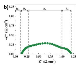
Fig. 2 (a) EIS analysis at different voltages for the AEMWE system using an AF1-HNN8-50 AEM and acid pretreated nickel electrodes: inset is the zoomed figure; (b) different resistances represented in a Nyquist plot, exemplarily at 2 V. Abbreviations: O, I, a and c stand for ohmic, interface, anode and cathode, respectively. Experimental conditions: 1 M KOH electrolyte on each side, 10 rpm flow rate and operation at 60 °C.
