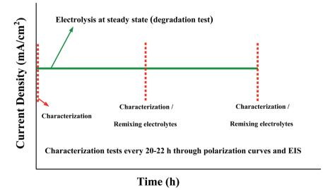
Fig. 1 The protocol for characterization and stability tests of the AEMWE system
