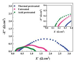
Fig. 3 EIS analysis of the AEMWE system using electrodes with different pretreatment methods at 2 V. Experimental conditions: 1 M KOH electrolyte on each side, a HNN8-50 Aemion™ membrane, 10 rpm flow rate and operation at 60 °C.
