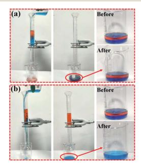
Fig. 10 Oil/water separation performance of the (a) ABS and (b) ABS-Ni membranes.
