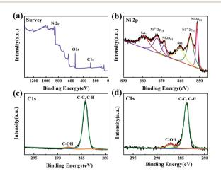
Fig. 7 (a, b) XPS patterns of the ABS-Ni membrane. (c, d) C 1s profile of the ABS and ABS-Ni membranes, respectively.
