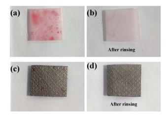
Fig. 8 Antifouling results of the (a, b) ABS and (c, d) ABS-Ni membranes
