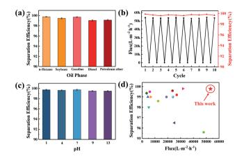
Fig. 11 Oil/water separation performance of the ABS-Ni membrane: (a) separation efficiency for different five oil/water systems; (b) separation efficiency in 10 cycles; (c) separation efficiency under different pH values; (d) comparison of separation efficiency.
