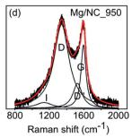
Fig. 3 Deconvoluted Raman spectra of the Mg/NC samples, pyrolyzed at different temperatures.
