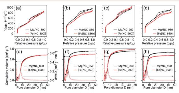
Fig. 2 (a)–(d)  $N_2$  physisorption isotherms on Mg/NC (black) and [Fe(N/C)] (red) samples, pyrolyzed at different temperatures. (e)–(h) Cumulative and differential pore size distributions (QS-DFT model)
