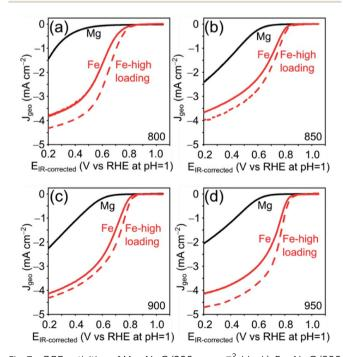
Fig. 7 ORR activities of Mg–N–C (200  $\mu$ g cm<sup>-2</sup>, black), Fe–N–C (200  $\mu$ g cm<sup>-2</sup>, red solid) and Fe–N–C (500  $\mu$ g cm<sup>-2</sup>, red dashed), following pyrolysis at four temperatures. LSVs in O<sub>2</sub>-saturated 0.1 M HClO<sub>4</sub>, rotating at 1600 rpm, scan rate 10 mV s<sup>-1</sup>.
