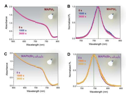
$\textbf{Fig. 4} \quad \text{MAPbI}_3 \text{ and MAPb} (Br_{0.18}|_{0.82})_3 \text{ light stability. UV-vis absorbance and photoluminescence spectra under continuous 1 sun illumination for the stability of the stab$ over 3600 s for (A and B) MAPbI<sub>3</sub> and (C and D) MAPb(Br<sub>0.18</sub>I<sub>0.82</sub>)<sub>3</sub>.
