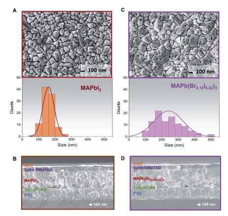
Fig. 3 MAPbl<sub>3</sub> and MAPb(Br<sub>0.18</sub>I<sub>0.82</sub>)<sub>3</sub> FESEM images. Top view, grain size distribution histogram (obtained over 100 grains), and cross-section FESEM images of (A and B) MAPbI<sub>3</sub> (brown) and (C and D) MAPb(Br<sub>0.18</sub>I<sub>0.82</sub>)<sub>3</sub> (purple).
